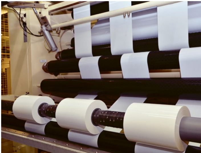
Manufacture of the Perlux® ultra product (left), with gel capsules (bottom left) and in the quality check (below)
