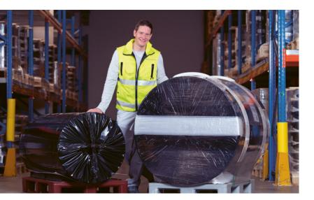
Philipp Gamma had the idea of doubling the length of the film on each mother reel. The new approach takes up less storage space and makes better use of transport container capacity. And it has reduced the associated transport costs by 15 to 20 per cent.
