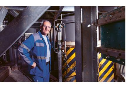
Sopi Gezim hit upon the idea of converting an existing secondary sorter into a further main sorter. With three main sorters, higher pulp volumes can now be processed at lower running levels. This has reduced the energy required per tonne of sorted pulp by 30%. The innovation has not only lowered costs: it benefits the environment, and has raised pulp quality, too.
